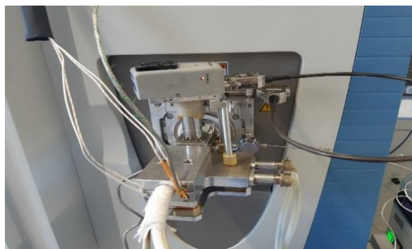
Figure 2: APPI source with its Body which is fixed to the orbitrap.
